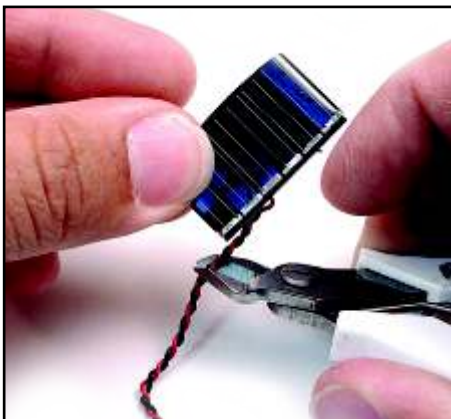
Clip off the wire 12mm ( \frac{1}{2} ”) past the long end of the solar cell.
