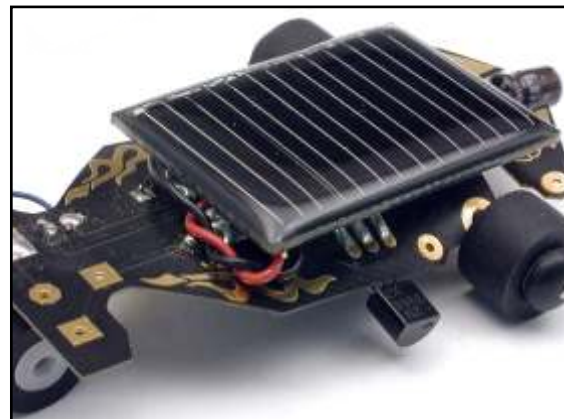
Strip the ends, and solder the solar cell back on. Doesn’t that look much neater now?
